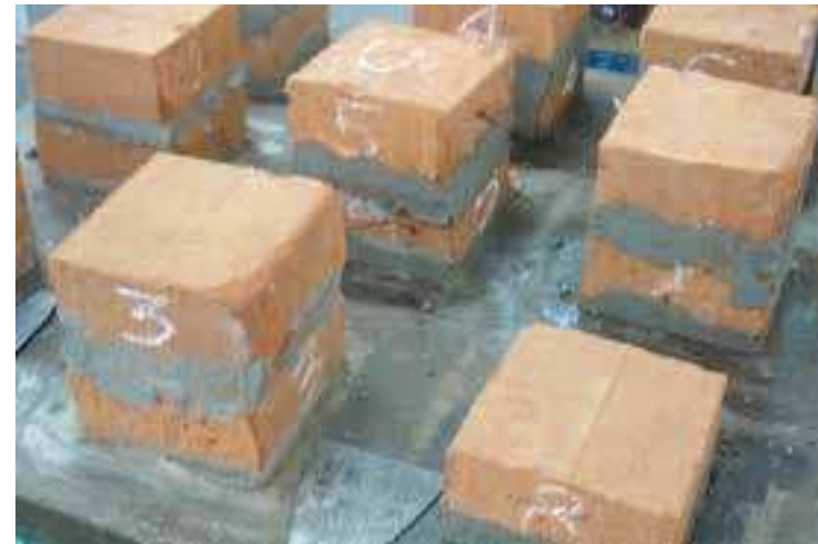
a) Fig.1 Samples: a) Cube; b) Cut adobe with the halves reunited (credits: Obede B. Faria, 2008)
