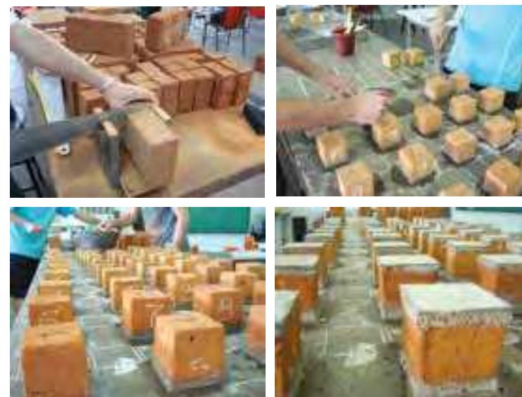
Fig.4 Some steps for the preparation of samples (credits: Obede B. Faria, 2008)
