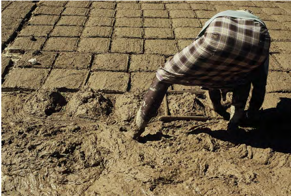
Fig. 5 – The quality of mudbricks is affected by the amount of water and straw, as well as the type of soil. In this commercial yard in Seyoun, brittle mudbricks result from a pea-soup consistency mud mix. (credits: Pamela Jerome, 1997)
