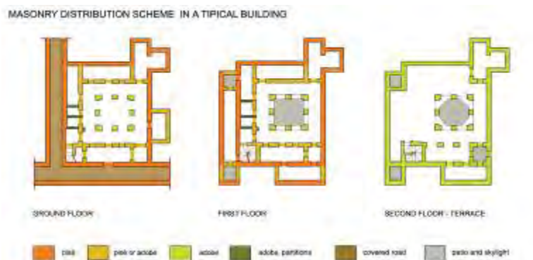
Fig. 1 – Scheme of the use of pisè and adobe masonry within a building. Case study of Hotel Dar Esseltane in Tissergat, Drâa Valley, Morocco. (credits: Baglioni E., 2009)
