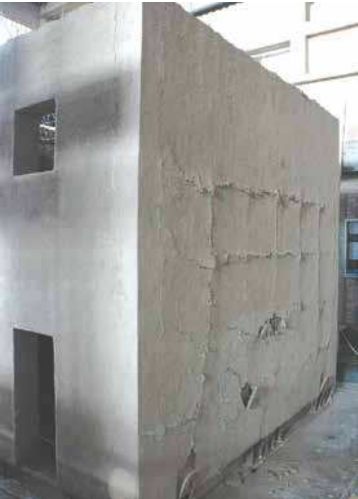
Fig.5 Detachments and cracks of the geogrid-reinforced plaster coating on the side perpendicular to the direction of the earthquake-movement simulation, after the fourth phase (displacement of 130 mm) (credits: Adell, 2008)
