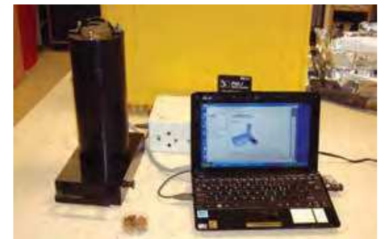
Fig.5 Portable luminescence-measurement apparatus comprising sample chamber with attached photomultiplier, control box, and laptop PC; sample in foreground (credits: Paul Adderley, 2012)
