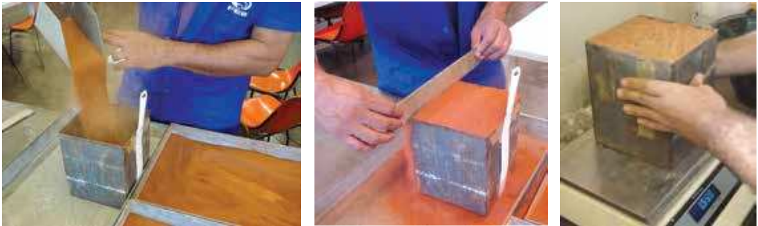
Fig.2 Determining loose soil density (credits: Obede B. Faria, 2008)
