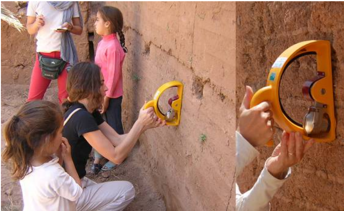
Fig. 4 – Sclerometer tests. (credits: Rovero L., 2007)
