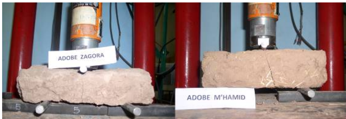
Fig. 3 – Sample F and G three point bending tests. (credits: Rovero L., 2009)
