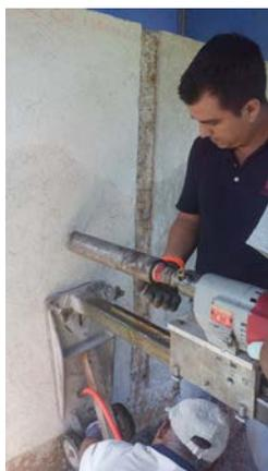
Figura 6. Ensayo de adherencia *pull-off*
