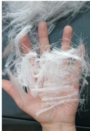
Figura 1. Fibra artificial fibratex de polipropileno
